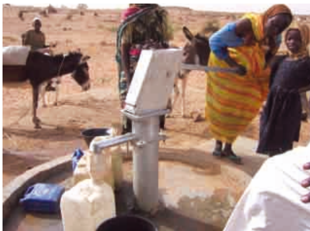
A well and a hand pump installed by SOLIDARITÉS in Darfur
